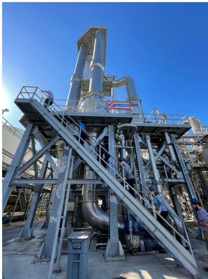
Tour attendees get an up-close perspective of a carbon reduction investment, the 94-foot tall evaporator, named Thor. This energy efficiency investment was supported by California Cap and Trade auction revenues. "The project would not have happened without the carbon reduction incentive," described Erick Watkins from Pacific Coast Producers.
